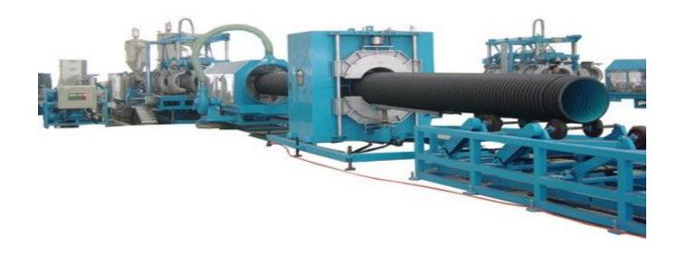
Process of forcing polymer through a shaped die, then cooled to form a pipe
