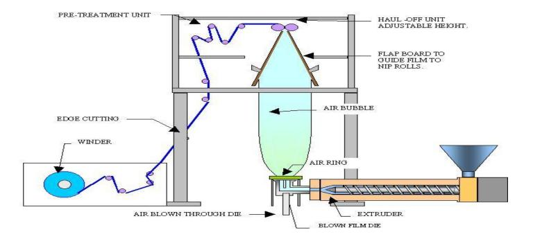
Film is processed when blowing air at the extruder die creates a tubular cross-section and is extruded through a spiral die, inflated, then drawn to the winding device.
