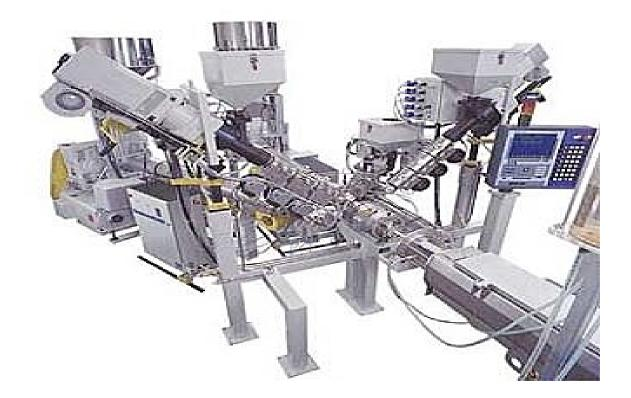
The process of extruding two or more materials through a single die with two or more orifices arranged so that the extrudates merge and weld together.
