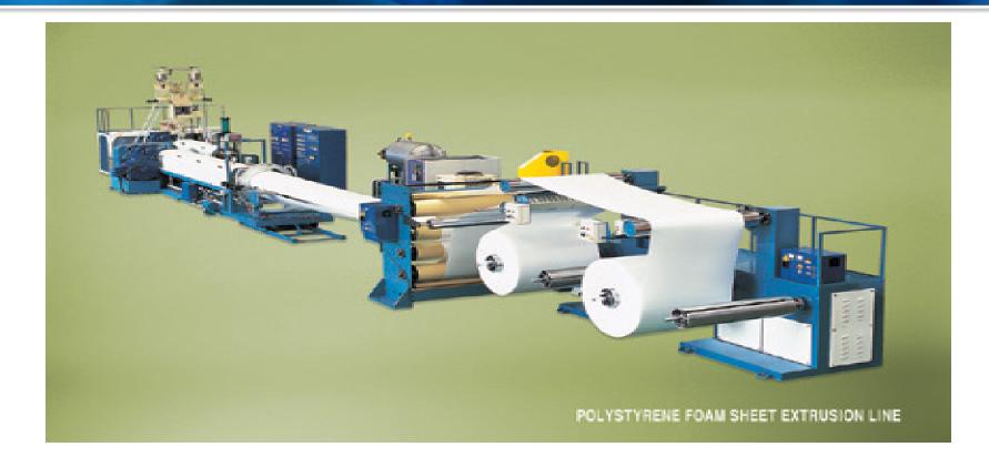
Plastic resin is mixed with chemical foaming agents and melted. The chemical foaming agent decomposes ,gas is dispersed in the polymer melt and expands upon exiting the die.
