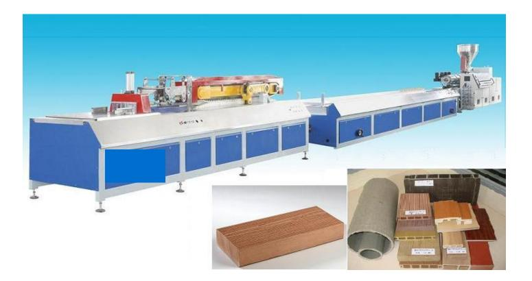
Plastic is forced through a die under heat & pressure to form a part with specific cross section.
