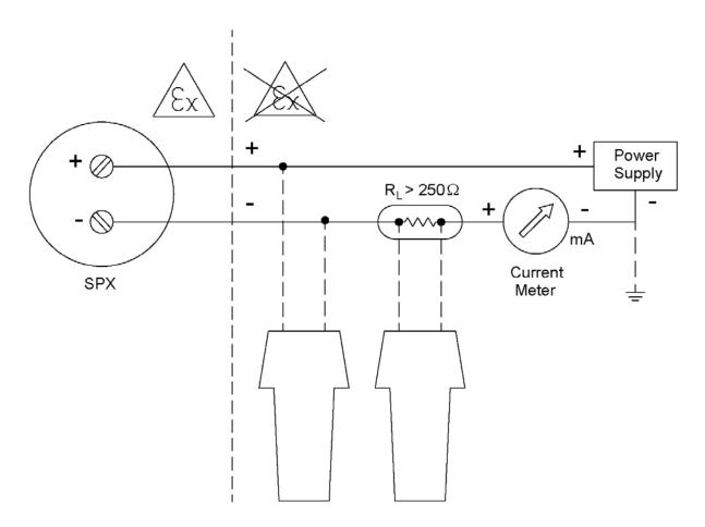
Figure 6-1 HART Communicator Interface
