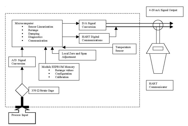
Figure 1-1 Block Diagram of Operation
