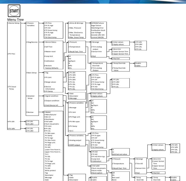
NOTE: Above is the Menu Tree for the latest Device Descriptor. For units with software revision < 100 refer to Appendix 2 for appropriate Menu Tree.
